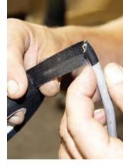
This tape is made of cloth backing that makes it durable and flexible with strong adhesion.
