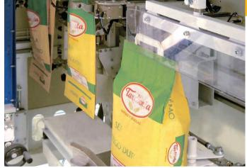
The vertical form fill seal machines are automatic packaging machines that begin by forming the plastic bags or standup pouches, simultaneously filling it with the intended product before the pack is sealed and cut.
